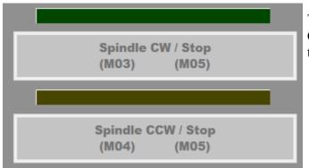
The Spindle CW / M05, and the Spindle CCW / M05 Are default toggle buttons for turning the spindle on and off.
