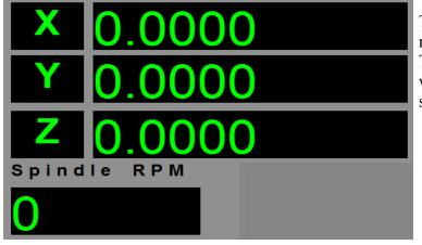
The DROS at the top left of the screen represent the current work coordinates. They are editable. The Spindle RPM DRO will display the current actual RPM of the spindle
