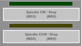
The Spindle CW / M05, and the Spindle CCW / M05 Are default toggle buttons for turning the spindle on and off.
