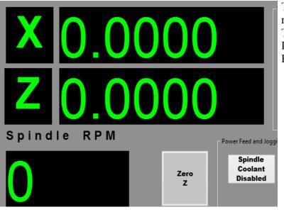
The DROS at the top left of the screen represent the current work coordinates. They are editable. The Spindle RPM DRO will display the current actual RPM of the spindle
