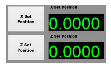
Setting up a manual move on a machine can be done in one of two ways. There are X, Y, and Z Set Position Buttons. The Machine should be either at or moved to the end position of the Manual Operation. Once the desired position is obtained, the appropriate Set Button(S) can be clicked and Mach will record the position to perform the Move.
