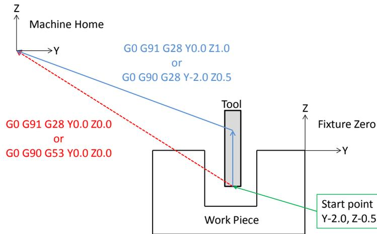
Figure 28-1: Zero return via intermediate point
