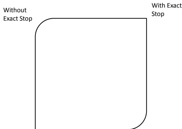
Figure 9-1: Square with exact stop on two corners
