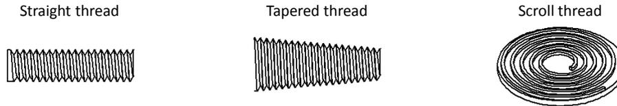
Figure 32-1: Basic thread types
