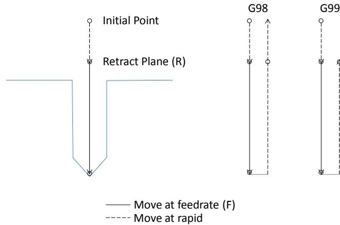
Figure 98-1: Initial and R point return setting.
