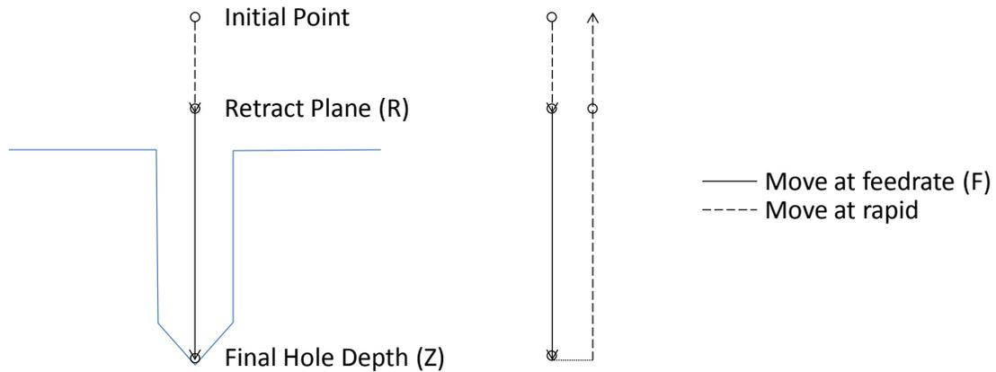
Figure 81-1: Motion of tool point for G81 cycle. End Z position will be determined by G98/99 setting.
