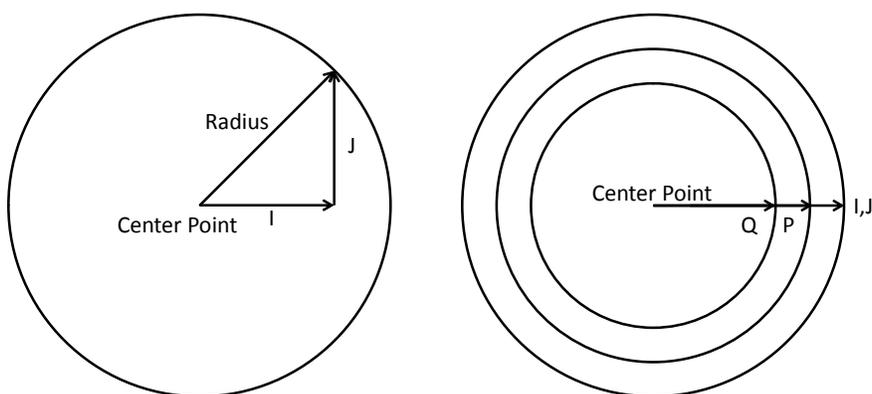
Figure 12-1: Tool motion during circle interpolation
