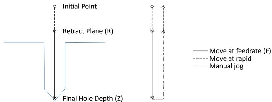
Figure 88-1: Motion of tool point for G85 cycle.
