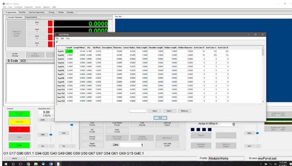
Next, you can enter in the dimensions of your stock by navigating to Configure>Plugins>Simulator-ModuleWorks. This will open a window that will allow you to set your stock and the bottom center position for your tool. This window is important and you may have to return to it to change these settings often.
