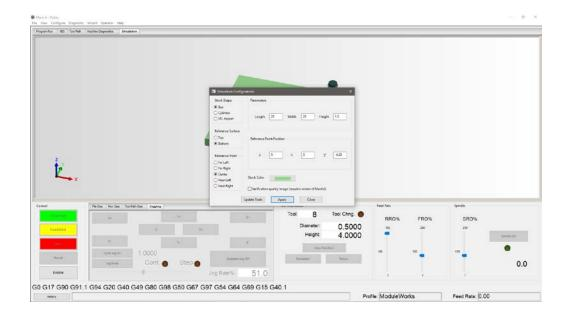
Once you have established your tool settings and configured your stock, navigate to the Simulation tab. You should see your tool and stock ready and waiting to be cut. Based on your cut file, you may have to maneuver your tool to the correct zero location. You can do this by accessing Configure>Plugins>Simulator-ModuleWorks and adjusting your Bottom Center Position so that your tool is in the correct starting location. (future changes coming)
