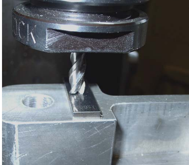
Figure 7.10 - Using a slip gage when touching Z offset on a mill
