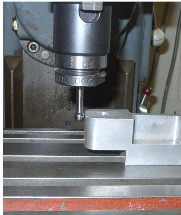
Figure 7.11 - Edge-finder in use on a mill
