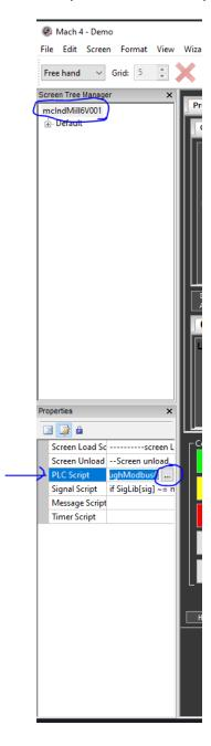
10. Copy and paste the code from the PLC.lua file (located in the examples directory of the Github zip file) into the PLC script. This code monitors the X axis position and sends the position to the Arduino via modbus. \*\*NOTE: be careful not to overwrite or delete anything in the PLC script, unless you know what you are doing.
