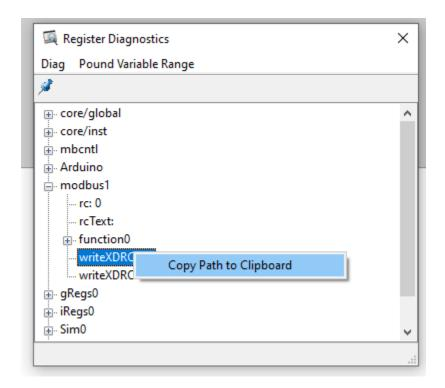
The register can be read to or written to from (the register path that was copied is placed in the quotes of the mcRegGetHandle function):
