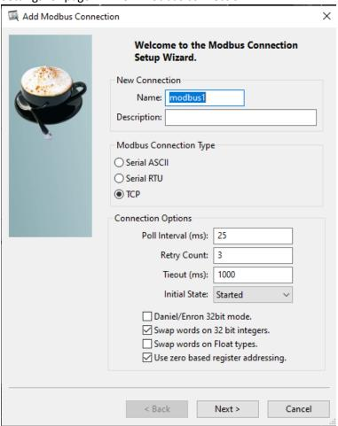
6. Settings for page 2 in new modbus connection. Enter the same IP address that was used in the Arduino sketch.
