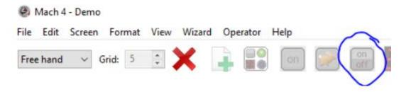
13. Select the Toggle button and edit the properties to map the output signal to the button.
