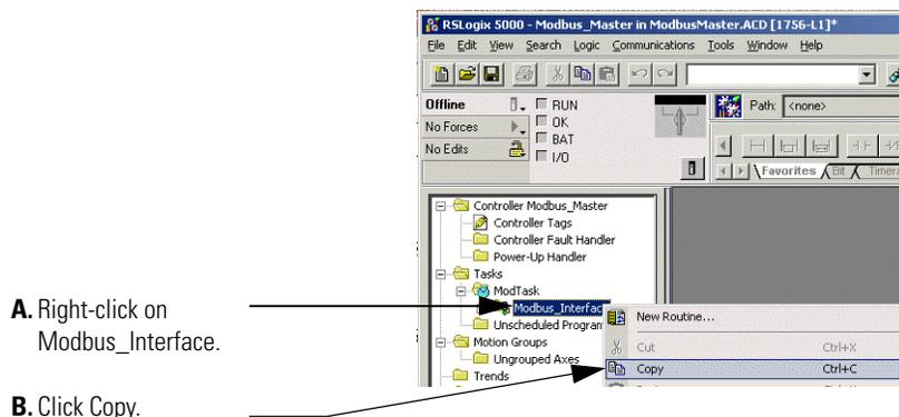
4. Paste the Modbus\_Interface program into the ModTask task in your RSLogix 5000 project.
