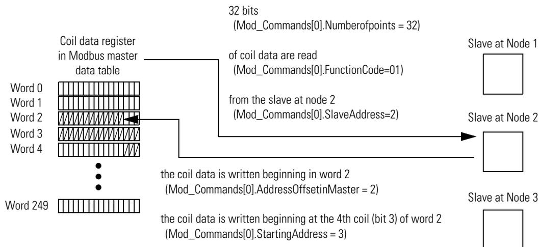
In this example, the Mod\_Commands[0].StartingAddress and Mod\_Commands[0].Numberofpoints tags represent bit values because the Modbus function code was 01 (Read Coils), a bit level code.
