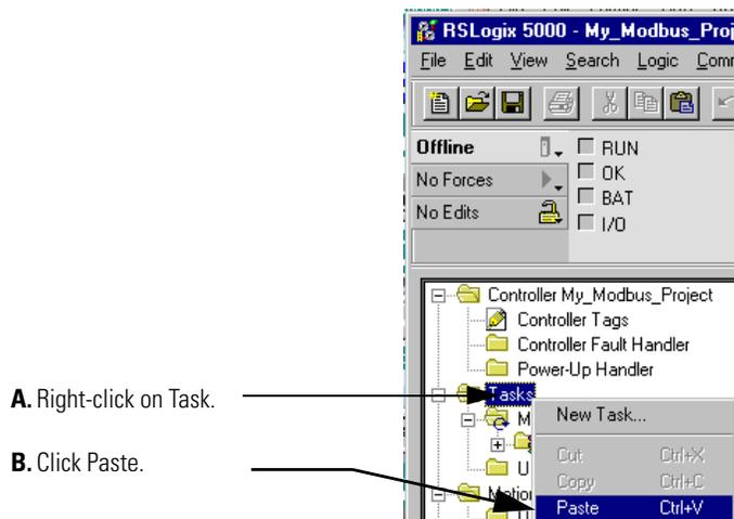
3. Copy the Modbus\_Interface program from the ModbusMaster.ACD file.
