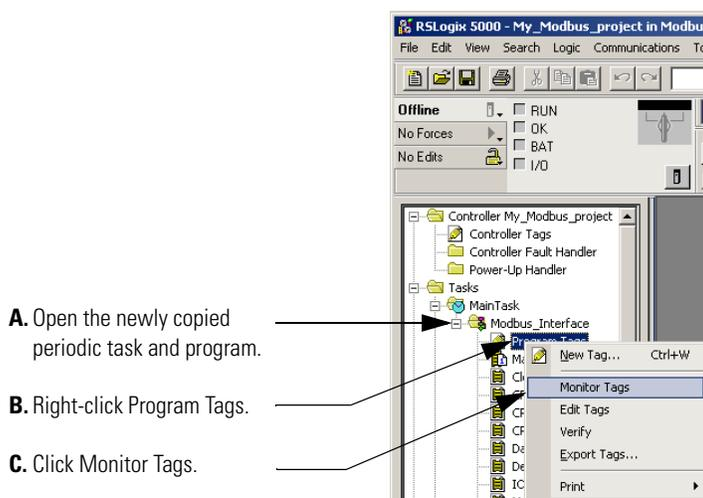
2. Scroll to the tags you need to monitor. The example screen below shows Mod\_Status tags used in the ModbusMaster file to monitor the operation of command element 1
