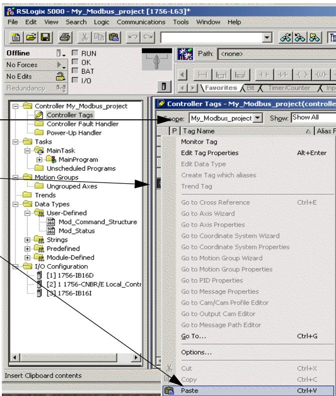
The image shows two screenshots of the RSLogix 5000 software interface. The first screenshot shows the project tree with 'Controller Tags' selected. The second screenshot shows the Tag Editor with a context menu open over the bottom tag line, and the 'Paste' option is highlighted. Arrows point from the text instructions to the corresponding elements in the screenshots.
