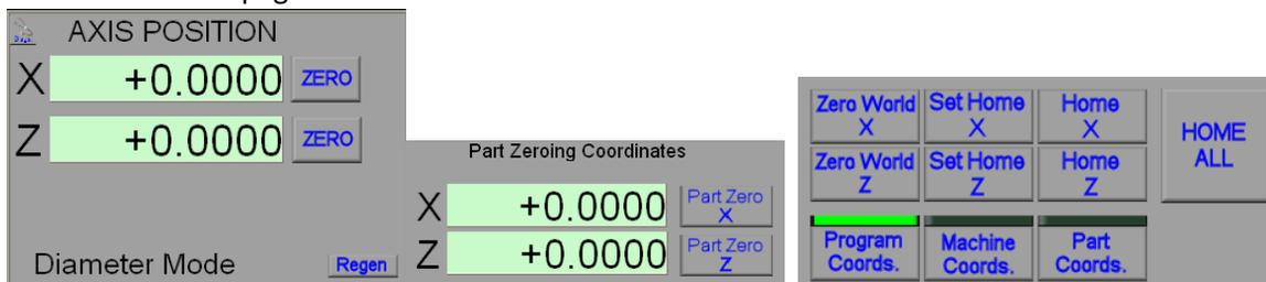
What is shown in the Axis Position DRO's depends on what coordinate system is selected and current mode. "Basically" PRC=PC when there is no G92 or G52 work offsets. PC includes any current Work offset and PC=MC ( which is in terms of radii ) if there is no Work Offset. PC is in terms of radius or diameter mode but MC X values are always absolute in terms of radii. Read the LM for complete definitions of the coordinate systems.
