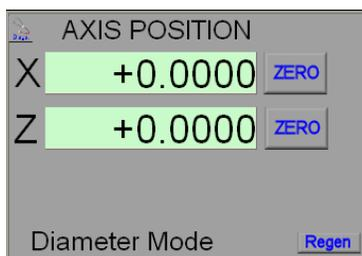
If one clicks the Zero World button it will zero the axis and also removes the current WO. Set Home will reference the axis. Once the machine is referenced MC axis definition is fixed in the controller and what you could do before no longer works. You can de-reference an axis but need to modify the screen to add a button.
