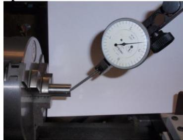
Indicate the rod so it is located on the lathe center, the rod should be parallel to the Z axis.
