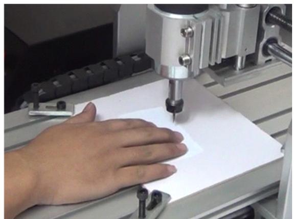
① First, we operate the XY axis through manual control, and move the principal axis close to the initial point; Install a flat base pointed knife.
