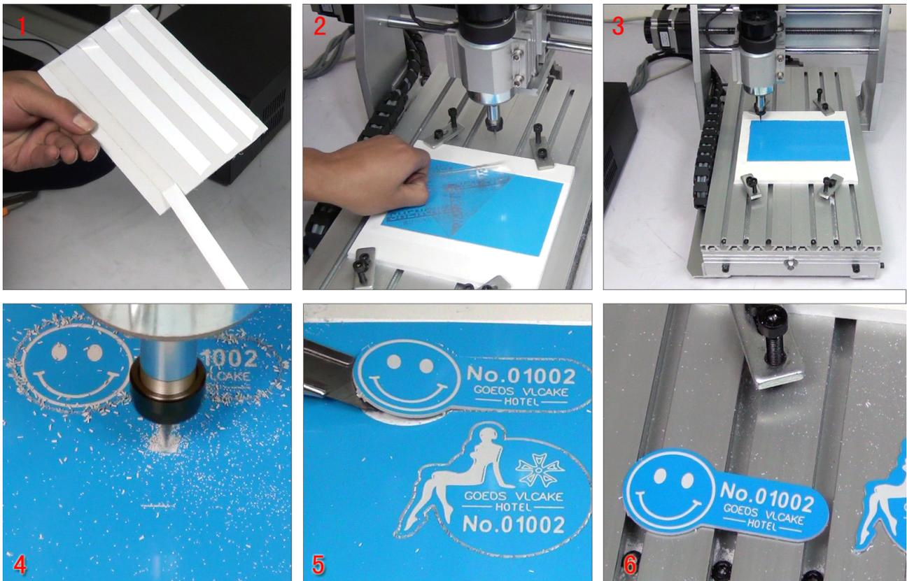
There is a file in the "tool path for machine test" of the random CD, with the file name of "shuangseban.nc". The area of this engraving file is about 75\*85mm. Because the double color plate is pasted on the auxiliary operating platform, the size of the material should within the scope of 90X90mm. Meanwhile, the initial point of this file is on the top left corner.
