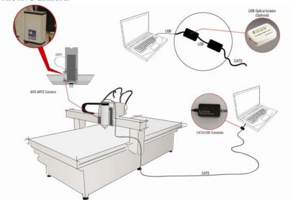
The actual AVS camera system is quite simple, it consists of a USB webcam that is plugged into the computer running the AVS App. Since typical USB connections are limited to about 5 meters and the USB cable itself is not suitable for the machine's cable tracks a CAT5/USB extender system is used as shown in the diagram. The CAT5/USB extender has a "receiver" that is plugged into the camera and a "sender" that is plugged into the computer.
