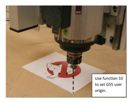
The next step is to set the G55 origin of the job close to the lower left corner of the sheet of paper. The reason you need to do this is so that the camera will get close enough to the first dot so that the AVS system can find it automatically.
