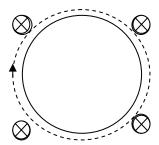
The dots must be sequenced first, before any of cutting contours. It does not matter the order of the dots as the AVS software will find the type A dot first, the type B second, and it really doesn't matter what the order of the rest of the dots is. It also will not matter what the depth of the drill is.
