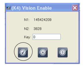
"N1" is a number that is unique to every A2MC. It is actually part of the MAC ID of the mini ITX computer in the A2MC. "N2" is the table ID of the machine.
