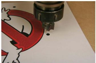
You can either use the jog keys to locate position 1 (P1) directly over a printed dot or you can drill a ¼ inch (6 mm) hole with position 1 (P1) into a white piece of plastic.
