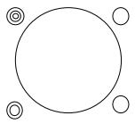
Note that the cut file is now a single large circle as this is the outline of the smiley face. The type C dots are simply small circles. Type A dot are three concentric circles and type B dots are two concentric circles.
