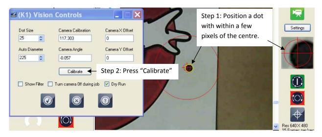
Calculating the camera calibration and the camera angle is done automatically by:
