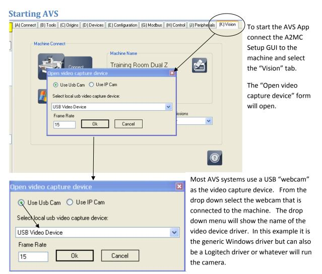
The frame rate can be set but is defaulted to 15 frames per second and it's usually best to just leave it at that speed. If you are operating on a very slow computer or a computer with a slow graphics card then you might have to slow this down in order to work. The AVS will still work but its performance will also slow down.
