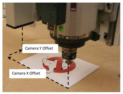
The camera X offset and camera Y offset is the distance from the centre of the tool in Position 1 to the centre of the camera image as shown on this diagram.
