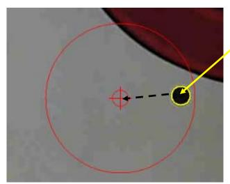
Once the tool inn P1 has been located the operator console will prompt, "Camera to P1 Mark". Return to the AVS software and use the jog features to move close to the dot that was marked.
