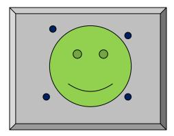
The dots should be black and about 0.25 inches or 6 mm in diameter. They should be well spread out. There should be at least three dots with four or five being optimal. The centre of these dots are then located by the AVS camera, processed by the AVS software which then adjusts the cutting file to exactly match the printed image.
