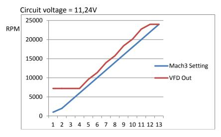
**Conclusion:** Keep working voltage to 10V to get 1:1 scaling, or else VFD output will be higher than mach setting, but at the expense of maximum VFD speed of course.
