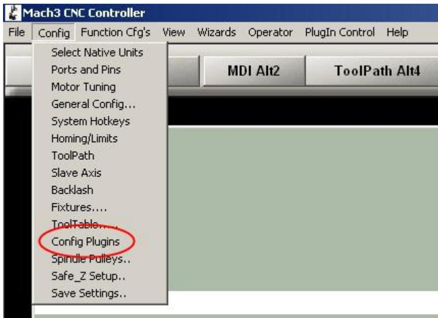
This will bring up a list of installed plugins. Locate the JoyPad plugin and enable it (marked as green V):
