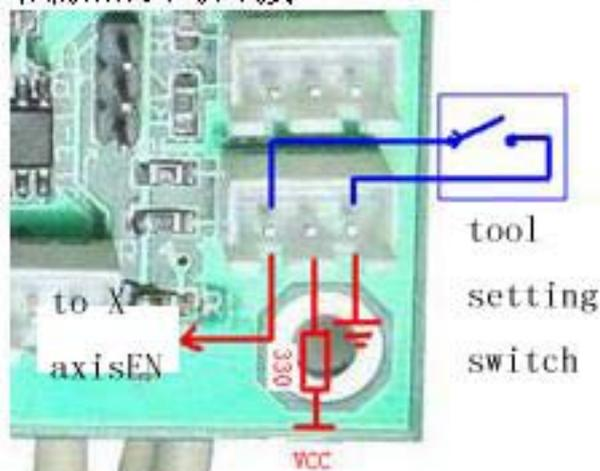
7.J13 is a 5-wire input port , it used for connecting other external equipments, the functions of the pin can be set up by the host computer software.
