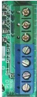
8.J14 parallel port P10 input signal connection jumper---P1-2 of the J14 closed , P10 connects to the P1of J13.
