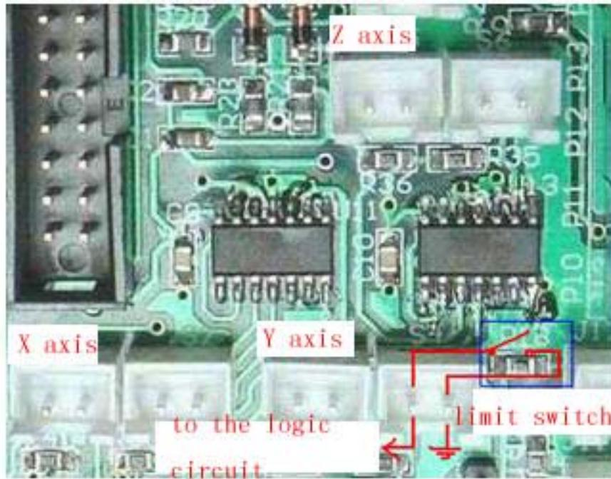
The limit switch connection: the limit switch is open normally, each axis has two switch.
