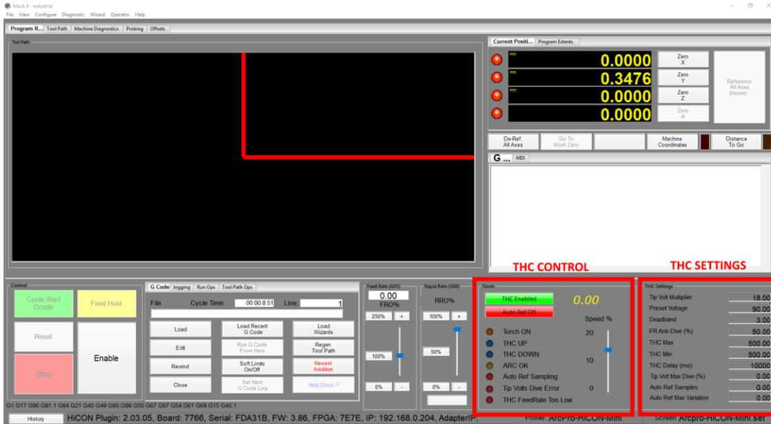
**THC Control** – This panel serves as the control interface for starting/stopping THC Mode (e.g. the automatic adjustment of the torch height while cutting).
