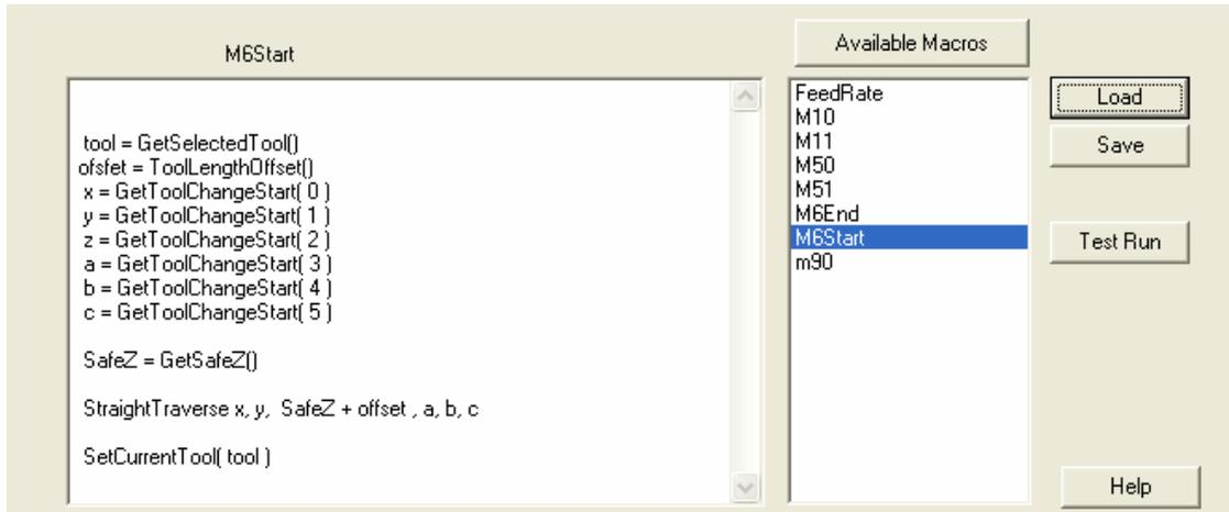
The Macros screen is used for editing, creating or testing a macro. The one you see in the picture is the macro used to start the tool-change process. It is Visual Basic Scripting.
