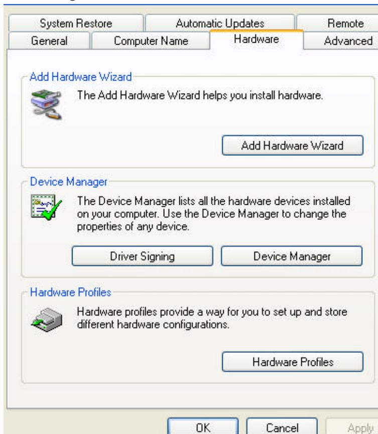
Select the hardware tab as shown and then hit the device manager button. A screen will appear with the following type of info. If you see a Master5 CNC Engines line, then a driver is loaded for Master5 or Mach1.
