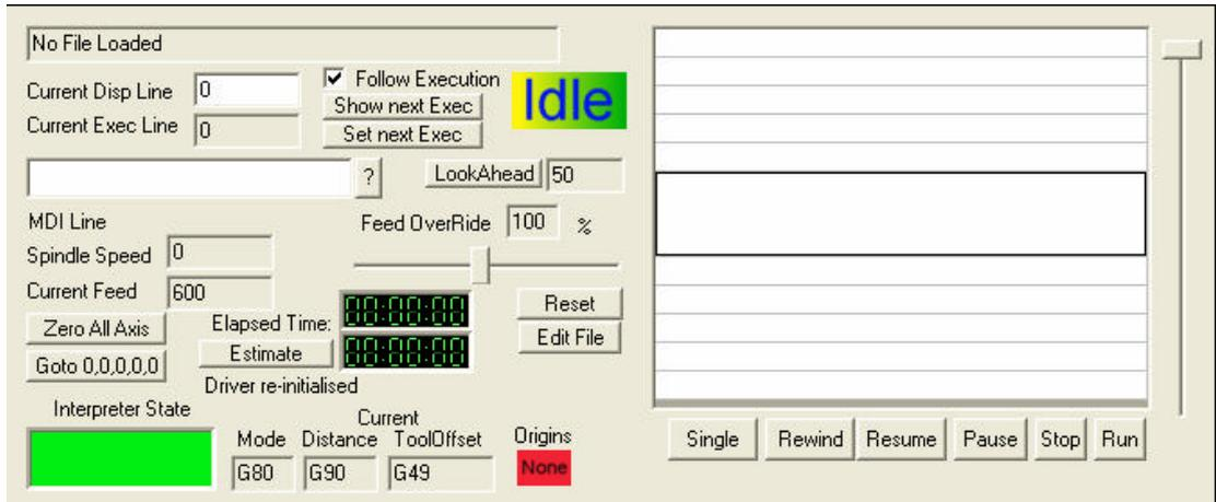
The top left box will display the name of any currently loaded G-Code file. Mach1 is a G-Code interpreter and all input filters, JPG, DXF, BMP, HPGL and others will create a G-Code file to be run. Input filters, when implemented will auto-load their G-Code output when creating a new file. The name of that file will be displayed here.
