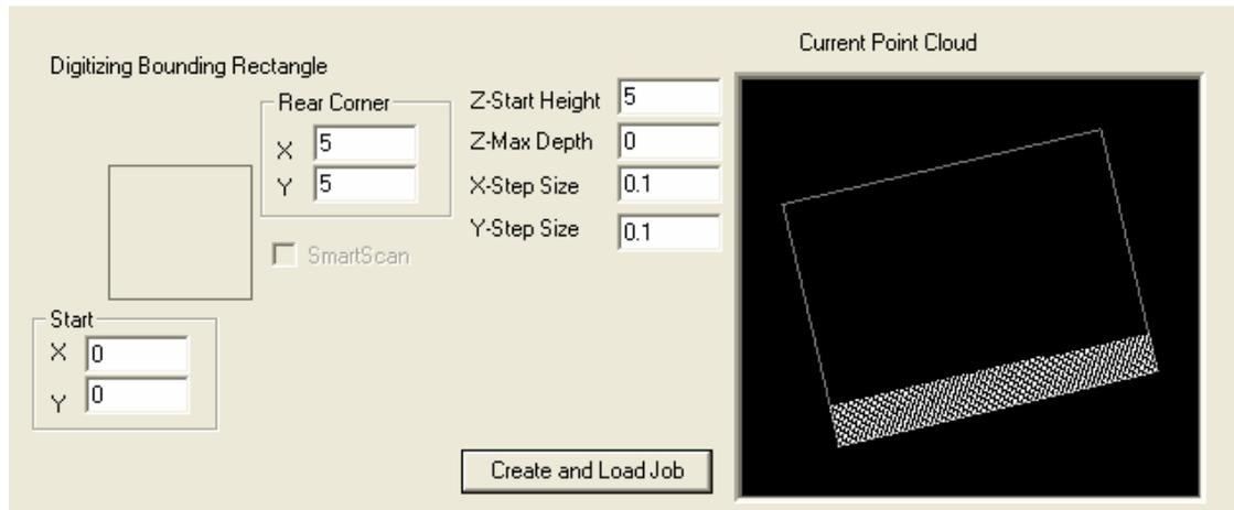
The digitize Wizard allows you to create a grid for digitizing. The start location is the 0,0,0 point of the grid, the rear corner is literally the rear corner of the digitizing grid. The step-over variables are how often to take a sample.
