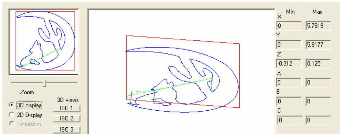
This display shows you your tool-path. The small window on your left is an overview window, it shows the complete job, the large window on the right is for detail zooming. By sliding the Zoom slider to the left you will see a black box get smaller. This is the display window into the detail box. Clicking and moving the mouse in the overview window will move the zoomed window around the job. The Green dashed lines are rapid moves while the solid blue lines are the feed rate moves.
