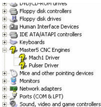
In this case the Mach1 driver is obvious. The Pulser Driver is for Master5 which can co-exist on the same machine. To remove the driver, just right click and select uninstall. It should go away immediately, if the system asks to reboot, then the driver locked up when running so you must be removing it because something went wrong. It may be corrupted so a re-install might help.
