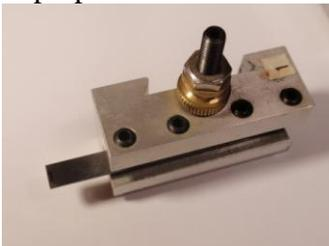
3. **Fix** the quick tool change **post** such that the face and end of the master tool are aligned properly with the reference rod. All other tools will be touched off to the same surfaces. All the other tools are adjusted in their holders to suite the cutting edges.
