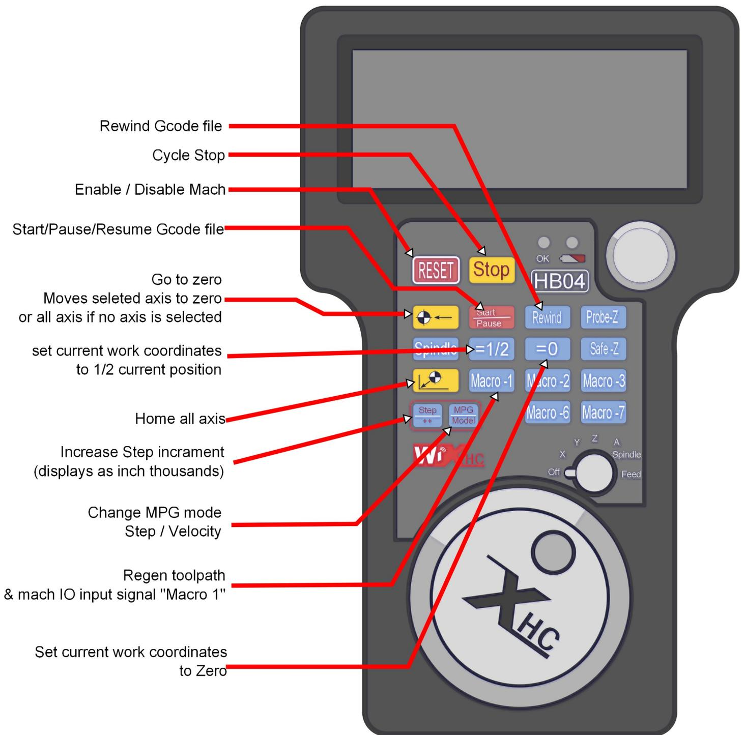
The following Buttons do not have functions but are instead mapped to Mach IO input signals:
