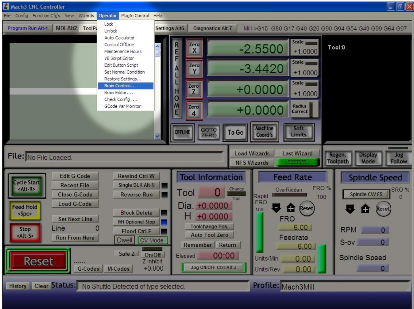
Now select the AnalogFRO.brn in the Loaded Brains window and click on the Enabled checkbox to enable it. In the end click on the button labeled "Reload All Brains" to activate it. You should be able to see the response of your FRO and SSO potentiometers on the Mach3 screen.
