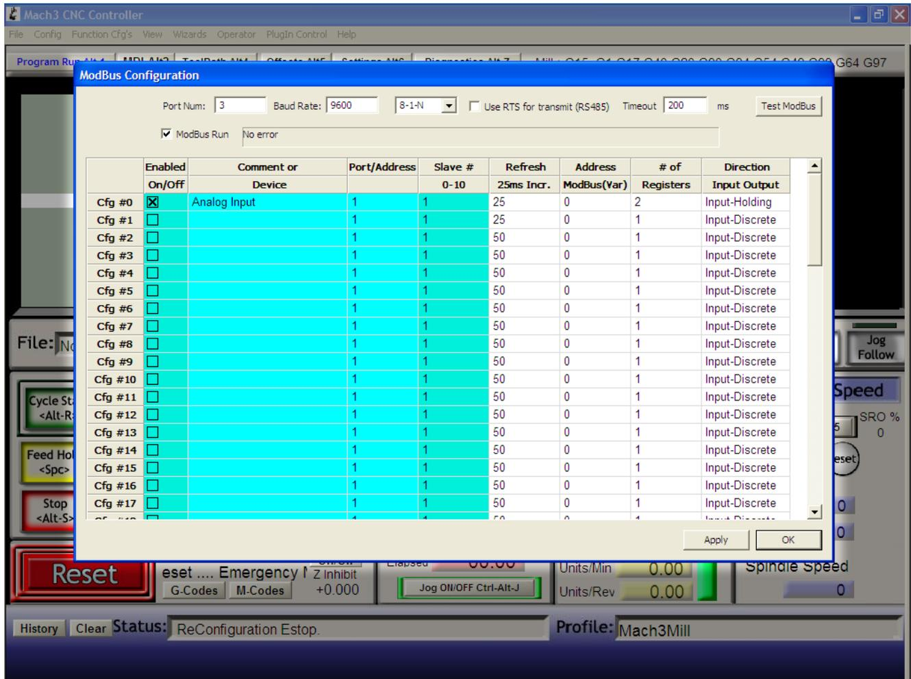
Please note the Port Num: might be other than 3 on your PC for the arduino. You can check the port number on which Arduino is installed in the arduino software. When you click on Apply button on this window the communication between Mach3 and Arduino should begin. You should see the TX and RX Led's on the Arduino board blinking at a rapid rate.
