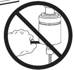
**Always** mount a torque bar to hold the tapping attachment's stop arm from rotating. The torque bar **must** be mounted securely to the table or quill of your machine. The torque bar installation **must** be stronger than the largest tap in the capacity range of your tapping attachment. Order Tapmatic Torque Bars shown.
