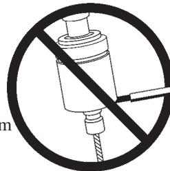
**Never** hold the stop arm by hand. On reversal, full power of the machine is transmitted through the stop arm and the operator could be seriously injured.
