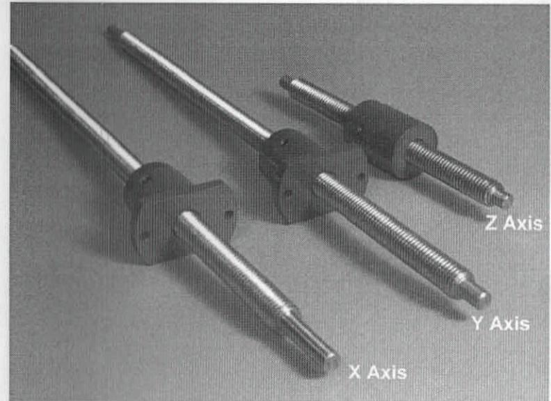
Panther CNC RouteR use new design to avoid above mentioned happen , we use screw without spring preload , low drag force and little lost capacity when spinning.
