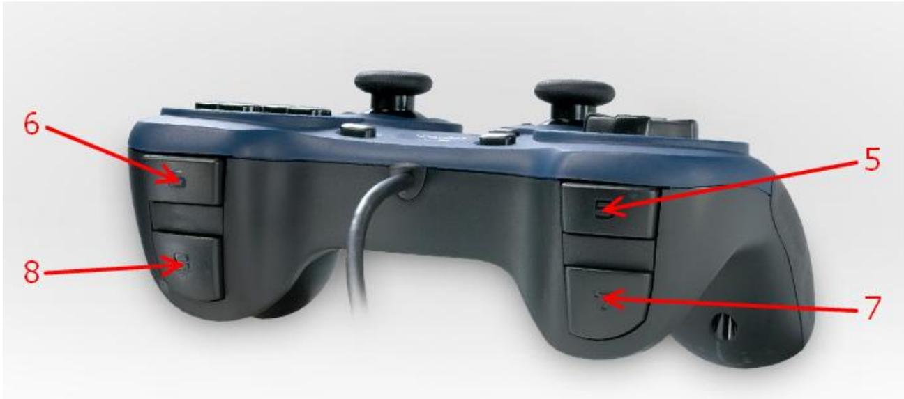
Button 5 and 6 is reserved as safety buttons and prevents the joysticks from operating when not pressed – this can prevent unintended movements of the machine in case the gamepad is dropped or operated by mistake.
