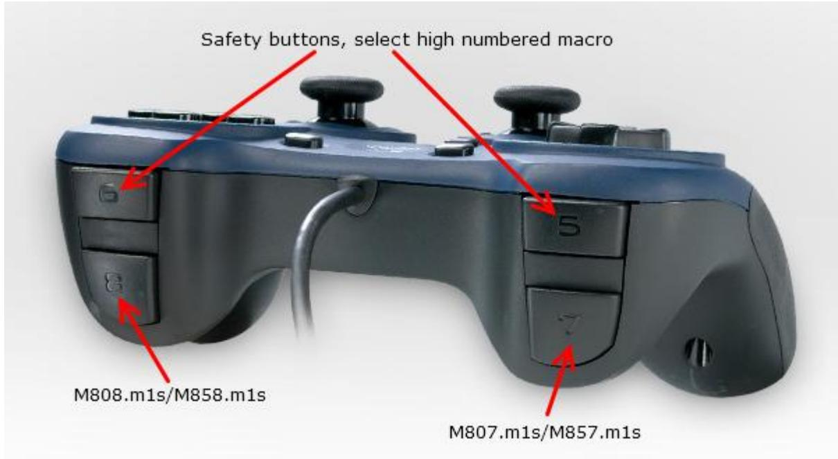
All macros can be executed in Mach3 as M-Codes, the macro M801.m1s will be executed if you type M801 in the command line or place the command in a G-Code file.
