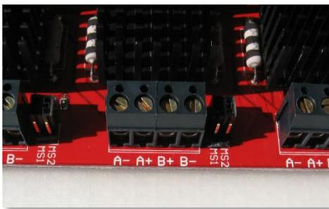
**Stepper Motors** with 4 wires is a true Bipolar motor and can only be used with a Bipolar control driver. Each of the two phase coils / windings have a pair of wires. Using a multi meter, you can identify the pairs of coils
