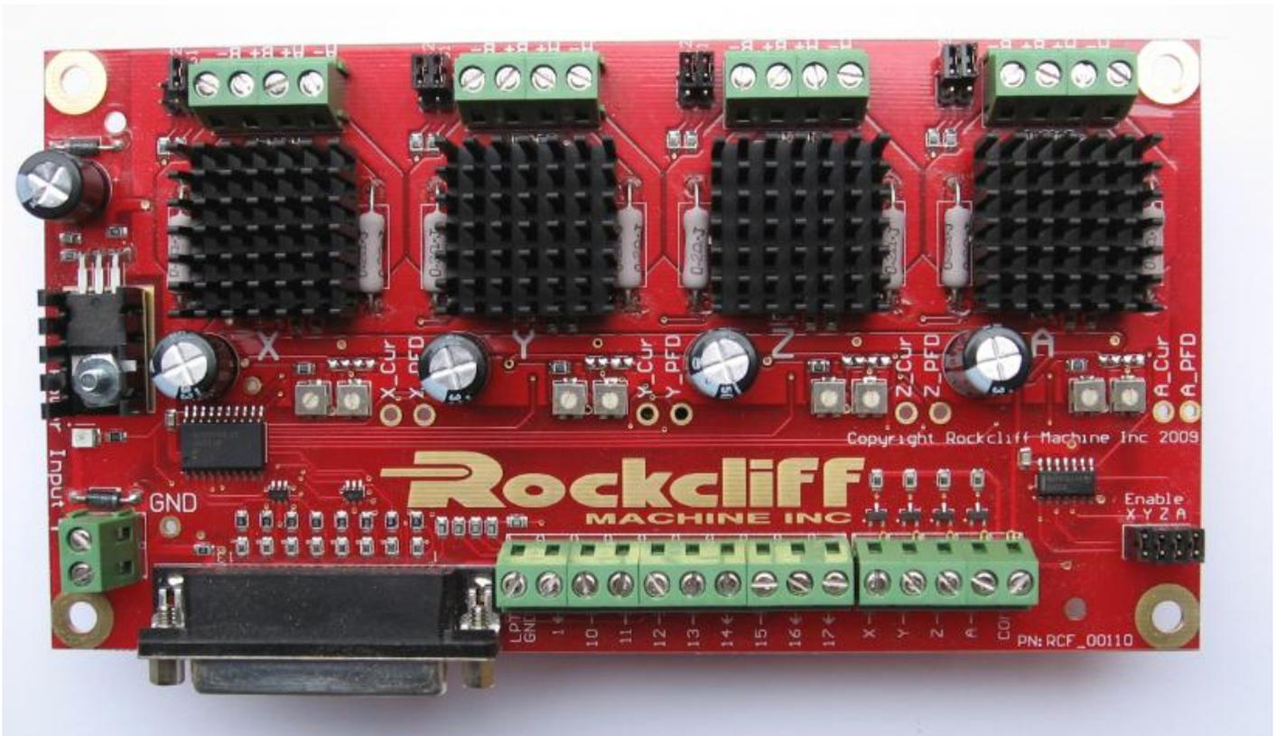
**Bipolar 4X Axis Micro Stepper Motor PWM Control A** Bipolar Motor Drives are by far preferred by most for best overall performance and compatibility, and with Pulsed Width Modulation Technology with give superior motor performance while running, and stay cooler while idle.
