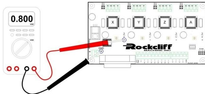
A voltage reading of 0.8 vdc is equal to 0.5 Amps to the motor
