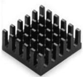
**Heat Sinks and Cooling Fans** Heat Sinks are provided for additional cooling to the motor driver IC chips, and power transistor, a heat sink should always be used when the current setting is set above 50% of the maximum setting.
