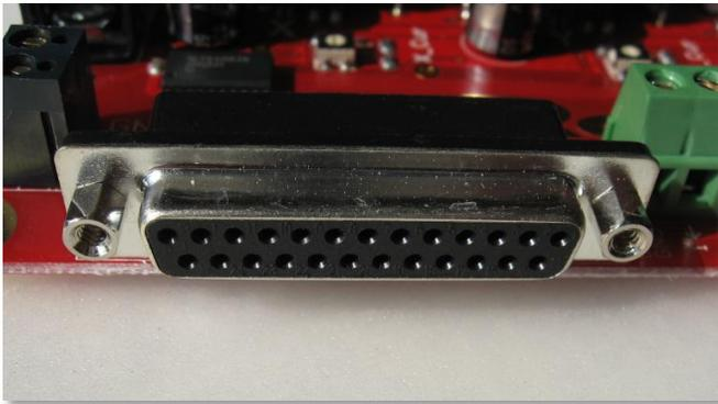
**Parallel Port (DB25 Printer Port)** connection cable used is a DB25 Cable straight thru male ended connector, the cable length should be as short as possible, and shielded, which will maximize signal strength and lower the chances of EMI (electro-magnetic interference), Most newer PC's do not install a DB25 port, but the use of a PCMCIA card in a laptop or a parallel port expansion card in a desktop is acceptable,
