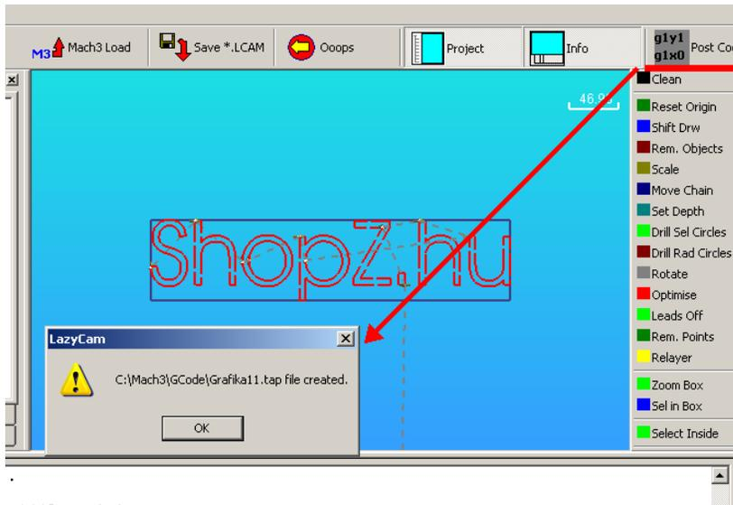
8. Go out of LazyCam or minimize, you may also want to save the file and Lazycam as an .LCAM for later retrieval. Here is the file posted into MACH.
