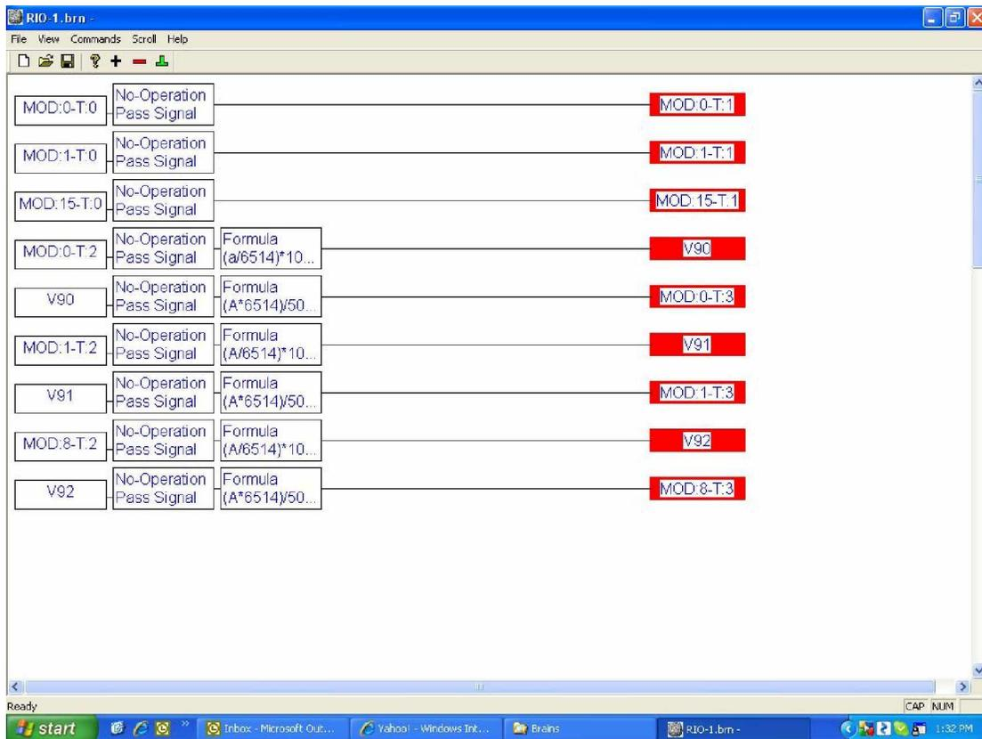
The above screen shows the sample brain file RIO-1.brn. It is showing the use of RIO digital inputs directly driving RIO digital outputs using the above configuration schemes. Of course, any Mach3 brain object may be substituted in place of either input or output to accomplish whatever task the user desires.
