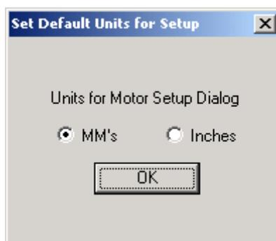
You can set Units as mm or inch.(Units for Foundertop CNCmachine is mm)
