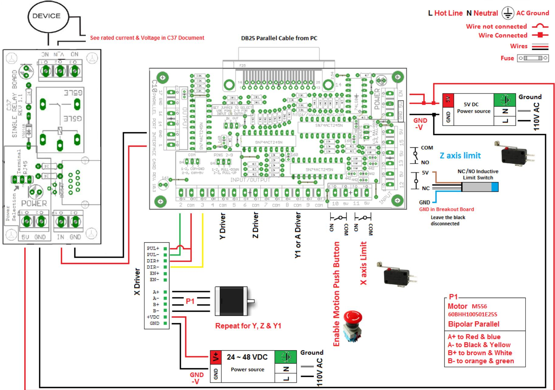
**Note Y1 and Y2 should be wired to Y pins in breakout board to change the direction of one motor switch phase A+ with A-
