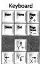
You can use to set up a 3-axis coordinate direction according to their needs, You can also refer to the above picture settings, In "Config—Ports and pins—Motor Outputs" settings, You can change the axis direction of change the "Dir\_LowActive" value.
