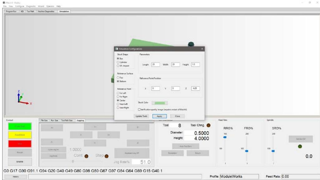
Once you have established your tool settings and configured your stock, navigate to the Simulation tab. You should see your tool and stock ready and waiting to be cut. Based on your cut file, you may have to maneuver your tool to the correct zero location. You can do this by accessing Configure>Plugins>Simulator-ModuleWorks and adjusting your Bottom Center Position so that your tool is in the correct starting location. (future changes coming)
