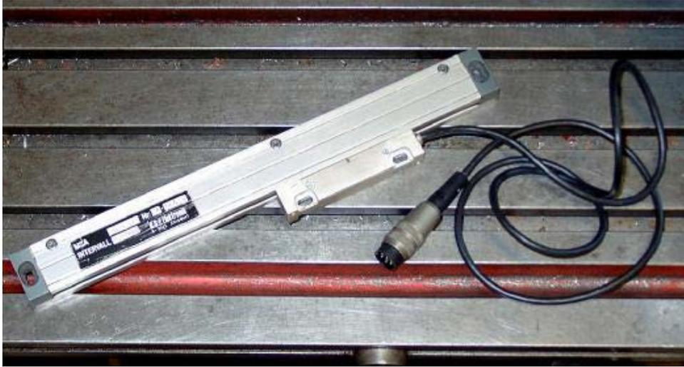
**Figure 4.15 - Glass scale encoder (awaiting installation)**
