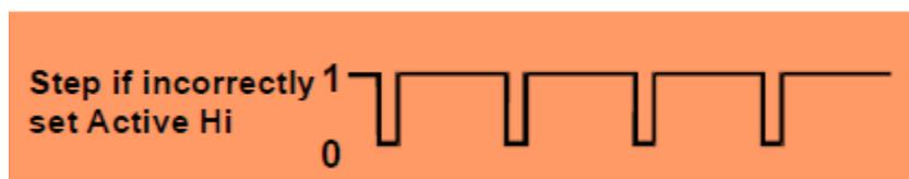
Figure 4.5 - Wrongly configured output alters step waveform
