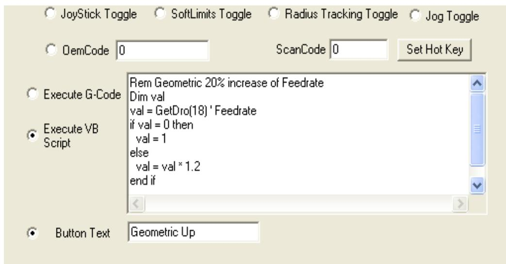
Figure 4.1 – Setting up the geometric feedrate button
