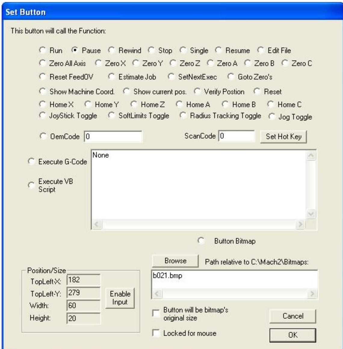
Figure 3.1 - Properties of standard Cycle Start button
