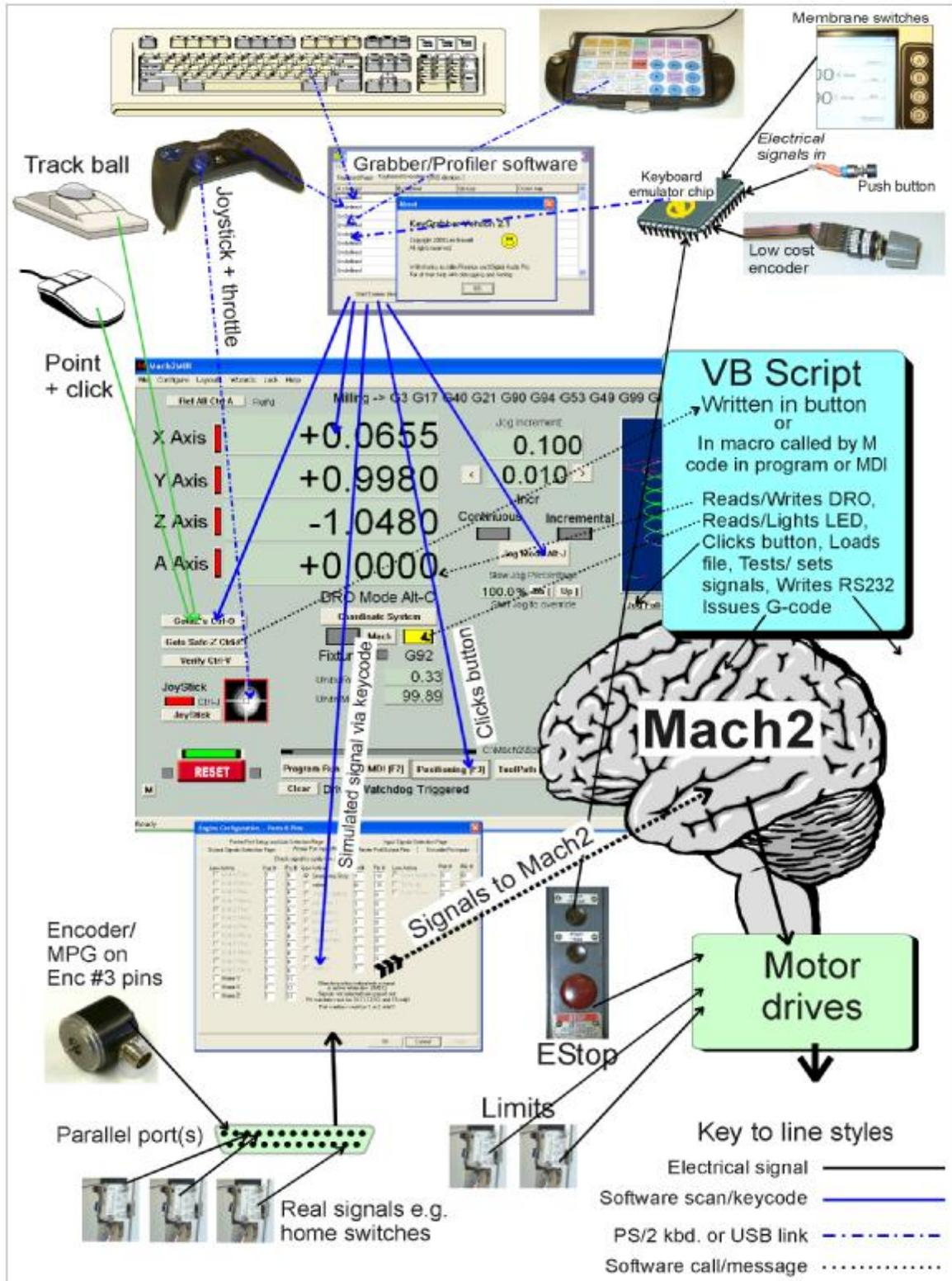
Figure 2.1 – Flow of control in a Mach2 system
