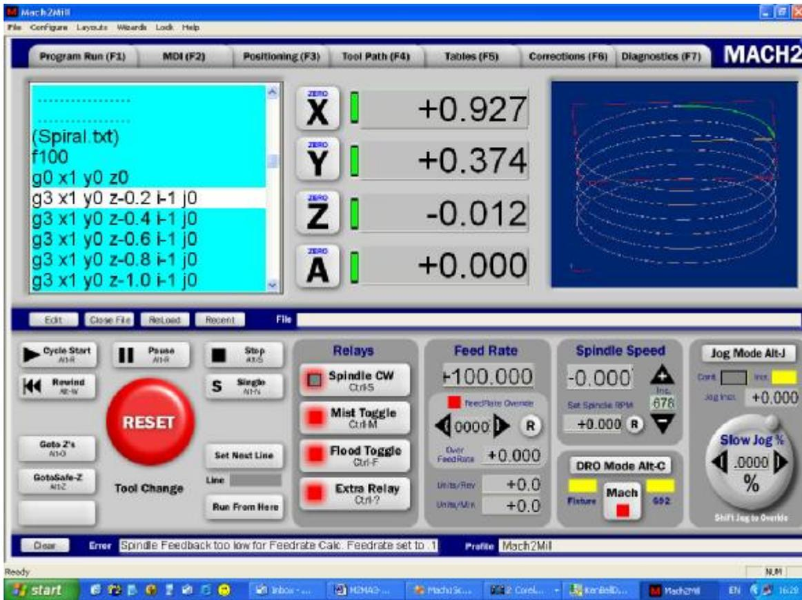
Figure 3.10 – Screen with all graphics on bitmap and transparent buttons
